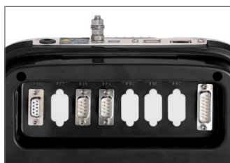
D-SUB connectors - IP40
